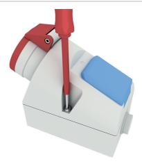
5. For variants without wiring: Create the necessary connections within the surface-mounting socket outlet according to one of the three possible connection options and test them. Tighten the screws on the connection terminals (7) with a torque of at least 1.2 Nm.
