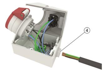
8. The terminals are open at the time of delivery. Guide the bare individual conductors into the opening (6) and tighten the screw (5) with a torque of at least 0.8 Nm. Take care to ensure that only the bare individual conductor (without insulation) is clamped. Pay attention to the
