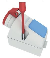
Loosen the screws on the contacts of the connection terminal and the screws (5) on the contacts of the three-phase outlet to which the cable is connected, and pull the individual conductors out of the terminals.
