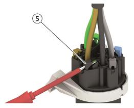
5. For surface mounting socket outlets and plugs: Pull out the cable from the housing and out of the cable gland (4).
