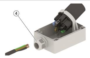
8. The terminals are open at the time of delivery. Guide the bare individual conductors into the opening near the contact slide (6) and press the contact slide (5) in the direction of the arrow to the side. The contact slide get latched and fixes the individual conductor. Take care to see that only the bare individual conductor (without insulation) is clamped. Pay attention to the marking of the terminals and ensure that the assignment of the individual conductors to the terminals is correct.
